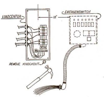
Identify an appropriate knockout to remove: 3/4" for the 6-circuit models and 1" for the 10-circuit models.
